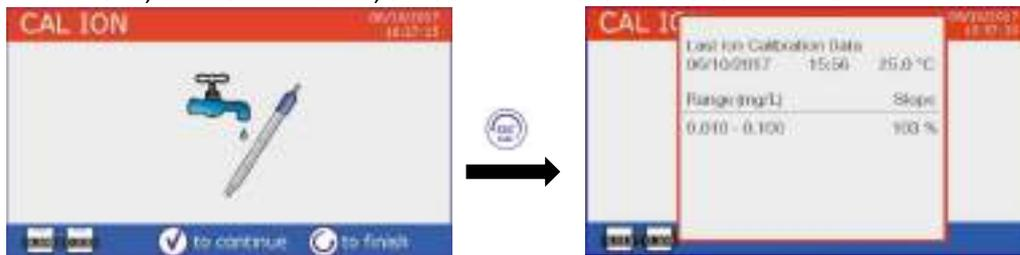
**Important:** carry out at least two calibration points; if you press
